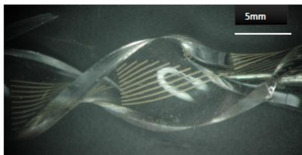
Figure 7. C-NCP electrodes fabricated via micromolding from PDMS filled with Ag nanoparticles<sup>38</sup>. Substrate has been twisted to show flexibility.
