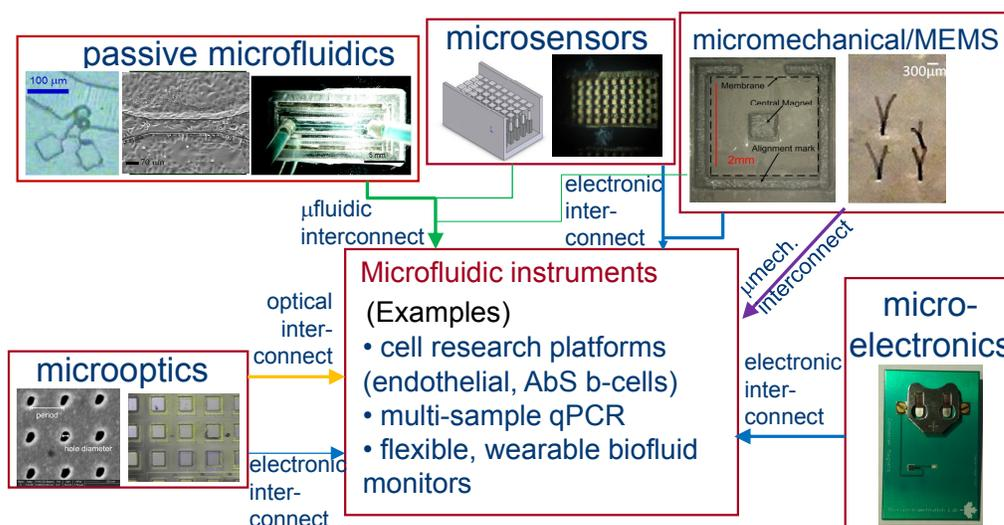
Figure 1. General conceptual microinstrument, showing potential subcomponent types, their required interconnect, and examples of functional microfluidic instrumentation that may result from the integration of these multiple subcomponents (similar to<sup>1</sup>).
