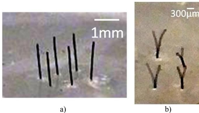
Figure 6. Magnetic composite polymer cilia: a) six cilia at rest; b) four cilia of different heights under a 7mT oscillating field<sup>35</sup>.
