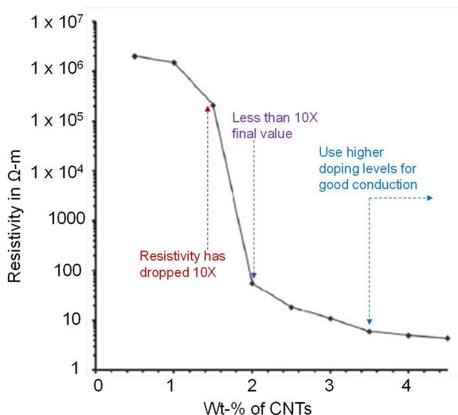
Figure 4. A typical (reversed) “S-shaped” curve for resistivity versus wt-% of nanoparticle filler in C-NCP (adapted from<sup>16</sup>).
