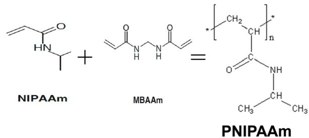
Figure 3. PNIPAAm hydrogel monomer and cross-linker<sup>6</sup>.
