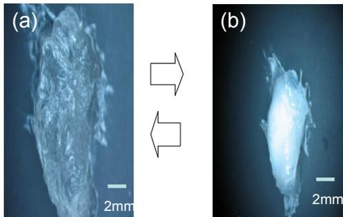
Figure 2. PNIPAAm hydrogel in: a) cooled, swollen state; b) heated, un-swollen state<sup>6</sup>.
