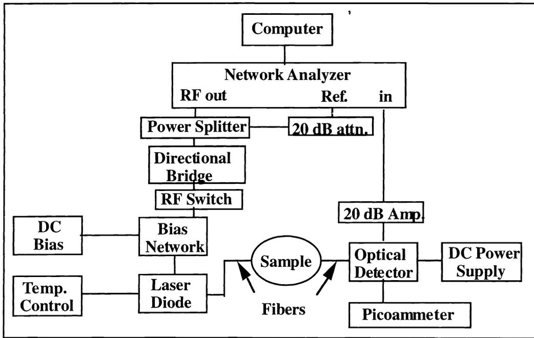
Figure 1. Schematic of the frequency-domain photon migration instrument.
