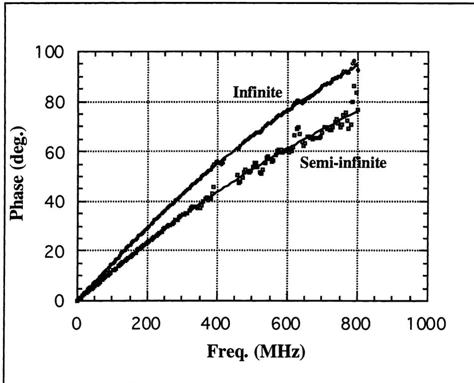
Figure 3. Phase vs. frequency response for 2% Intralipid and 1  $\mu\text{g/ml}$  NiSPC tissue-simulating solutions of two geometries. In both cases, the effective source-detector separation was 7.0 mm. The curves represent best fits to the data.
