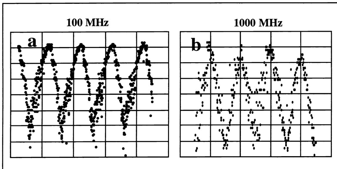
Figure 2. Source modulation at a dc bias of 254 mA and a) 100 MHz and b) 1000 MHz. The vertical scales in a) and b) are 100 and 50 mV/div. respectively. The corresponding horizontal scales are 10 and 1 ns/div. respectively.
