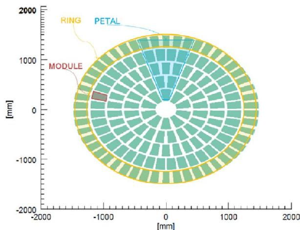
**Fig. 2.** Design of an entire mirror system using an arrangement of modules made of glass segments. Each of these 150 modules holds between 40 and 100 single glass sheets.
