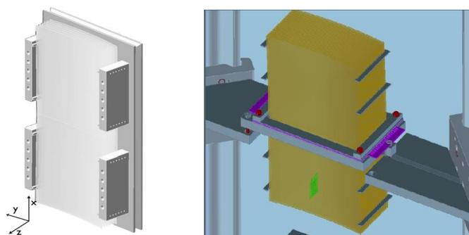
Fig. 6. Model of current 8-point mounting system (left) and new central based integration system (right)
