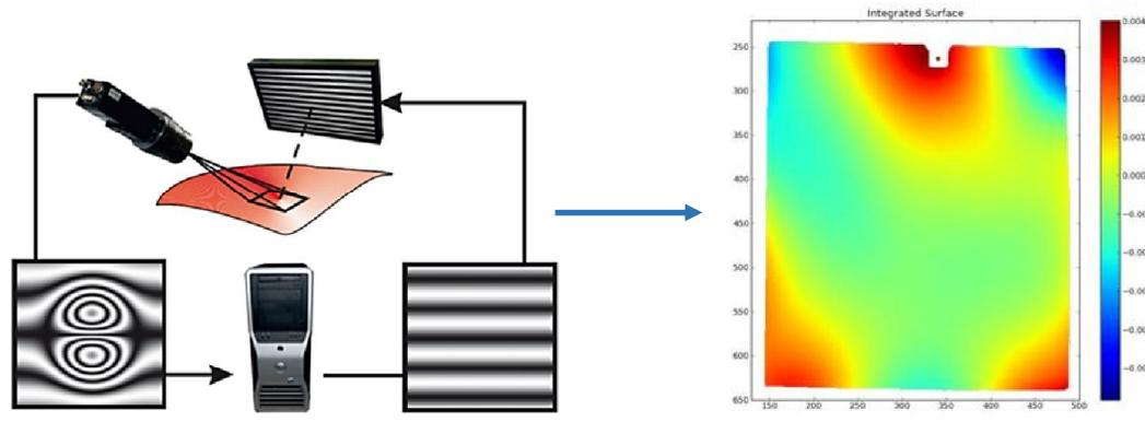
**Fig. 5.** Schematic view of the deflectometer to measure deformations in the glass. The picture on the right is a real measurement of a deformed surface due to glue influence.
