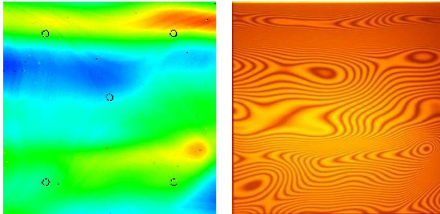
**Fig. 4.** Comparison of glass thickness measured by optical sensor (left) with double beam interference pattern (right) using sodium light. This glass has a peak-to-valley thickness variation of  $10\mu\text{m}$ .
