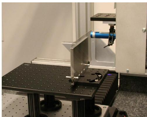
**Fig. 4.** 3D-precision table in MPE clean room with chromatic optical sensor
