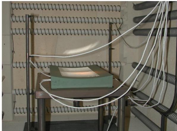
**Fig. 3.** Slumped glass in the MPE lab oven. The intersection line between parabola and hyperbola is clearly visible.
