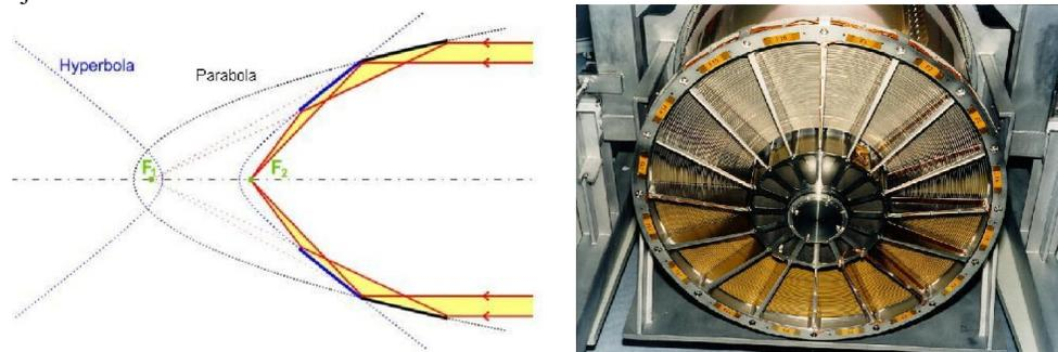
**Fig. 1.** Left: Wolter-I system for reflecting X-ray optics; right: one of the three X-ray telescope mirror modules of the XMM-Newton, launched in 1999. Each mirror module consists of 58 Wolter-I nested shells, designed to optimise the effective area
