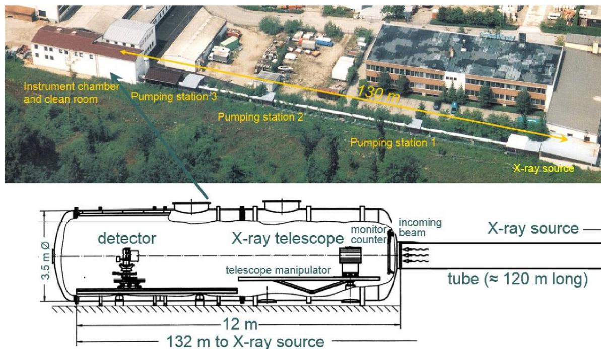
Fig. 7. PANTER X-ray testing facility. The lower panel shows a detailed schematic view of the instrument chamber.
