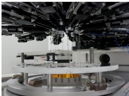
**Fig. 8.** Measurement of single shell performances on AVOB
