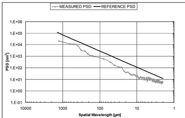
**Fig. 3.** One-dimensional PSDs compared with eROSITA reference PSD
