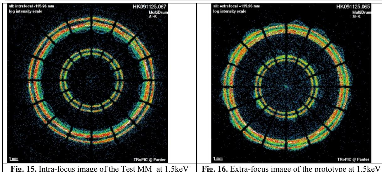
**Fig. 15.** Intra-focus image of the Test MM at 1.5keV
