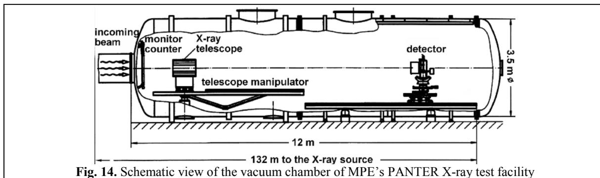
Fig. 14. Schematic view of the vacuum chamber of MPE's PANTER X-ray test facility
