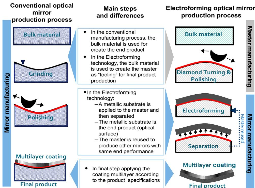
Fig. 2. Electroforming process
