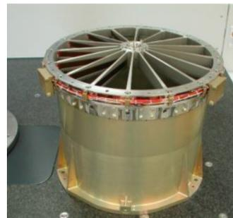
**Fig. 13.** Mirror module ready for shells integration
