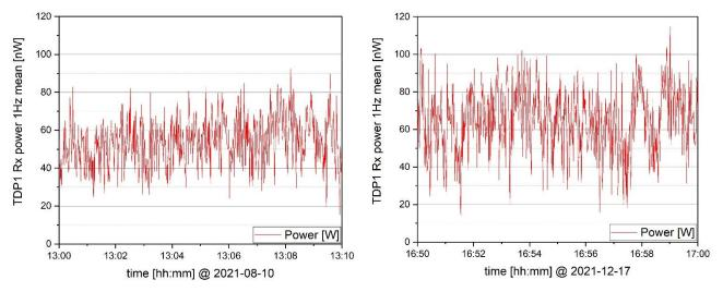
Figure 6. Receive power performance (1 Hz calibrated mean) for Zimmerwald (2021-08-10) and Tenerife (2021-12-17).
