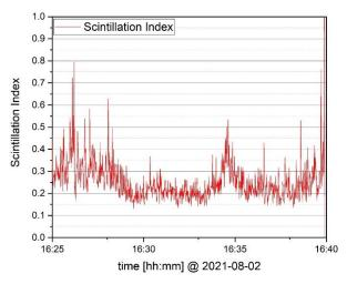
Figure 7. Scintillation Index of a link from the T-AOGS at Zimmerwald to TDP1-LCT at 2021-08-02 16:20.
