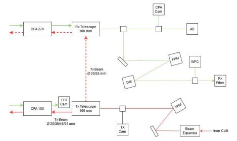
Figure 2. Receive and Transmit path of the T-AOGS.
