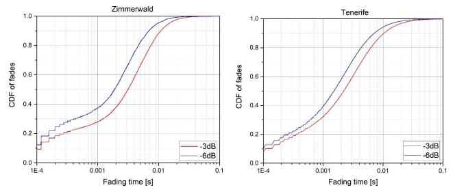
Figure 8. The cumulated density function of the number of fades relative to the fade duration at the GEO LCT for Zimmerwald (left) and Tenerife [5] (right)
