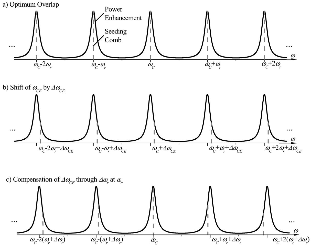
Figure 2. Illustration of the effect of a shift  $\Delta\omega_{CE}$  of the carrier-envelope offset frequency  $\omega_{CE}$  on the enhanced frequency comb, if the laser-cavity lock is realized by controlling the repetition frequency  $\omega_r$  such that the central optical frequency  $\omega_C$  is locked to the peak of a cavity resonance.
