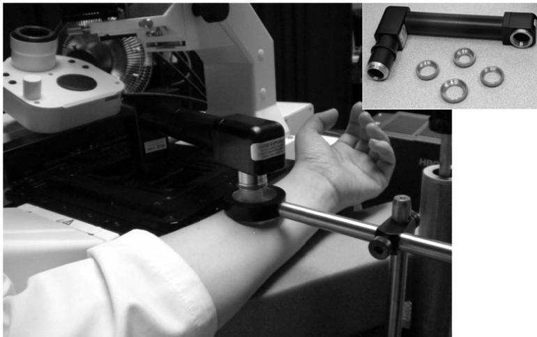
Fig. 3. Microscopy set-up for *in-vivo* TPEF imaging and spectroscopy measurements. Insert (top right) shows the objective inverter used.
