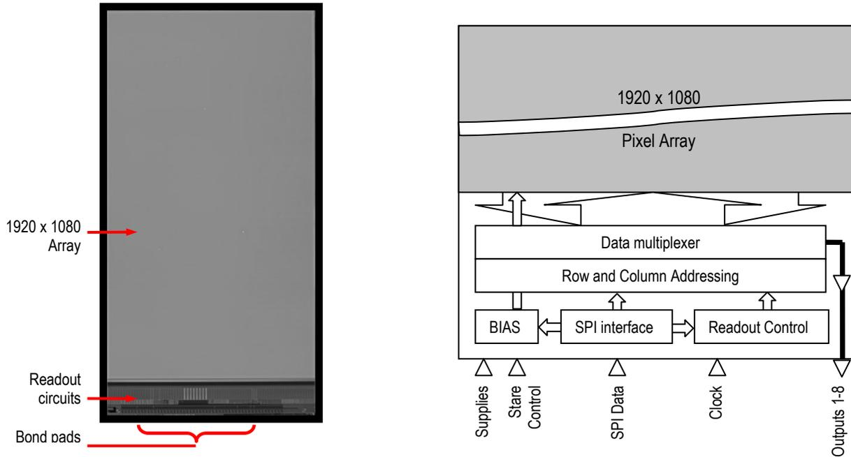
Figure 7 Photograph and architecture of FALCON HD
