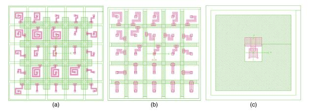
**Fig. 1** Layout of (a) main, (b) enhanced, and (c) UHR MMC sensors. The Au:Er sensor (green shaded), Au thermal links (red shaded) between sensor and x-ray absorber support stems, and Au x-ray absorbers (green open) are shown. Absorber size is 50, 25, and 50  $\mu$ m, respectively, for main, enhanced, and UHR sensors, whereas the overall hydra unit cells shown have sizes 250, 125, and 50  $\mu$ m.
