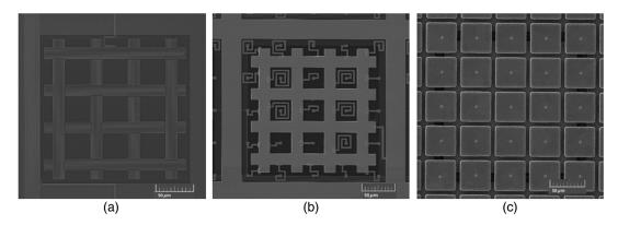
**Fig. 9** Evolution of a main array hydra sensor during fabrication. (a) Sensor meander coil laid out in a waffle shaped pattern. (b) After deposition of Au:Er, heat sinking grid and hydra thermal links. (c)  $5 \times 5$  hydra of 2.8- $\mu$ m thick electroplated Au absorbers suspended over sensor. The overall hydra size is 250  $\mu$ m × 250  $\mu$ m.
