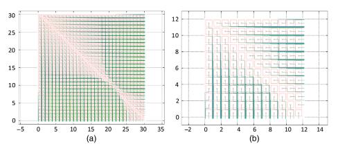
Fig. 4 Topological wiring schemes for one quadrant of an  $N \times N$  sensor array for (a) N = 60 or (b) 24.
