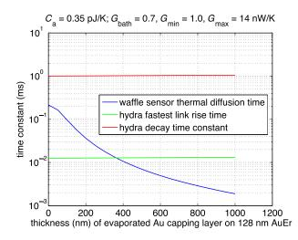
**Fig. 2** Calculated thermal diffusion time across the Au:Er main array waffle sensor as a function of the thickness of a pure Au capping layer added to speed thermalization. The thermal diffusion time (curve) is compared with the fastest expected hydra pulse rise time (lower horizontal line) and the overall hydra decay time constant (upper horizontal line).
