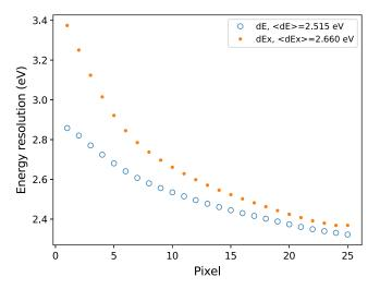
**Fig. 11** Simulation predicting the FWHM energy resolution of the  $5 \times 5$  hydra sensor with 800-nm pitch meander coils in the MMC main array in LXM. The energy resolution without errors in position correlation is dE, whereas dEx includes the effect of uncertainty in determining the x-ray absorption location in the  $5 \times 5$  hydra for an x-ray energy of 200 eV. For x-ray energies much larger than 200 eV, the energy resolution approaches dE.
