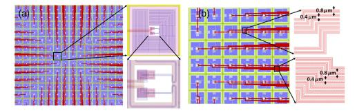
**Fig. 7** (a) LXM UHR array sensor design with successive close-ups of one Au:Er annular sensor plus the top level Nb sensor coil that meanders to fill the area under the Au:Er annulus, and the interconnection to lower wiring layers, through vias near the center of the sensor, to a twin-microstrip wire pair and ground plane. (b) Details of the Nb wiring in lower level muntins, which are shielded from the main array wiring and sensors by the intervening ground planes.
