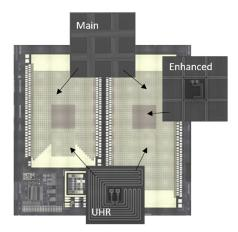
Fig. 8 Die layout of prototype MMC LXM array. The 22 mm  $\times$  22 mm reticle is divided into two chips differing only in size. Insets show locations of main array, enhanced array, and UHR array pixels.
