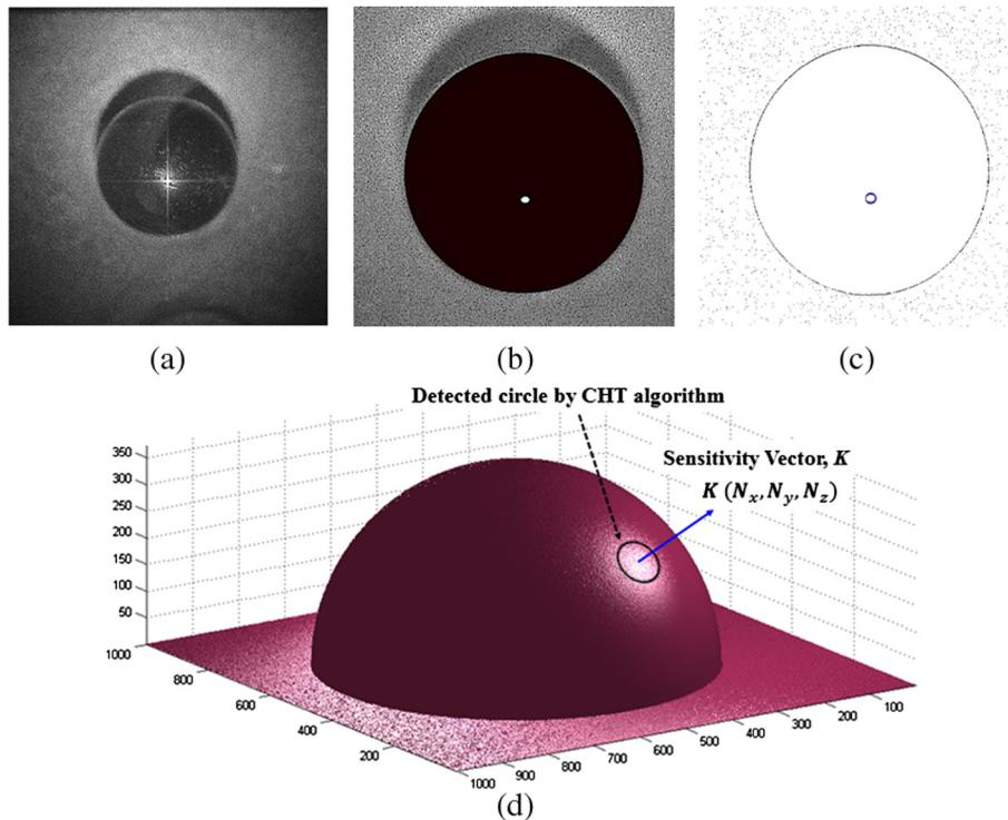
**Fig. 7** Automatic determination of a sensitivity vector by use of a specular reflective sphere and circular Hough transformation (CHT): (a) image of a specular reflective sphere illuminated with one of the object beams, (b) cropped, enhanced image of the sphere, (c) CHT algorithm is used to detect the specular highlighted area and its centroid, and (d) the normal vector at the centroid of the detected highlighted area defines the sensitivity vector.
