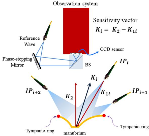
**Fig. 4** 3-D displacement measurements of the TM surface by the method of multiple illumination directions. Sensitivity vectors for each illumination direction,  $K_i$ , are obtained by vectorial subtraction of the corresponding unit observation vector,  $K_2$ , from the unit illumination vector,  $K_{1i}$ . The geometry of the TM limits the maximum angle of illumination that can be implemented to achieve a well-conditioned sensitivity matrix.
