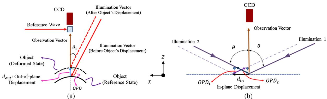
**Fig. 5** Two displacement measurement schemes that are combined to achieve 3-D displacement measurements in the hybrid method: (a) configuration for out-of-plane (along  $z$ -axis) displacement measurements and (b) configuration for in-plane (along  $x$ - or  $y$ -axes) displacement measurements. The dashed lines represent illuminations after displacement occurs. OPD is OPL difference.
