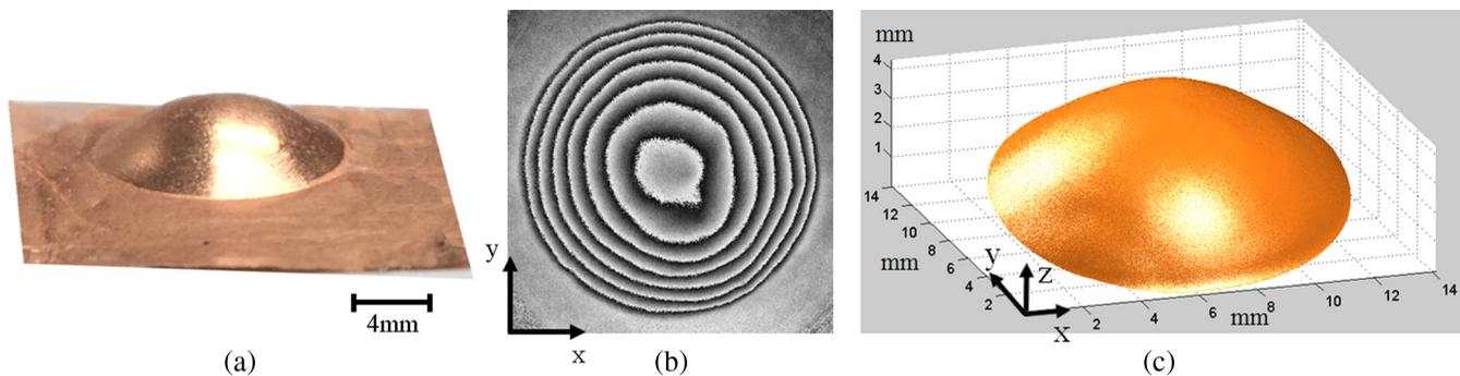
**Fig. 8** Measurements of the shape of an artificial membrane using dual-wavelength holographic contouring: (a) semi-spherical membrane with a thickness of  $25 \mu\text{m}$  and a radius of  $6 \text{ mm}$ , (b) wrapped optical phase corresponding to the shape of the membrane, and (c) 3-D scaled shape of the membrane.
