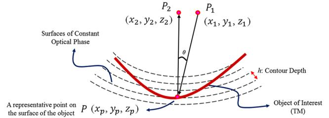
**Fig. 3** Optical path length (OPL) of the laser light in dual-wavelength holographic contouring.  $P_1$  is the point of illumination,  $P_2$  is the point of observation, and  $P$  is a point on the surface of the object of interest. Surfaces of constant optical phase intersect the object of interest generating contours of depth  $h$ .
