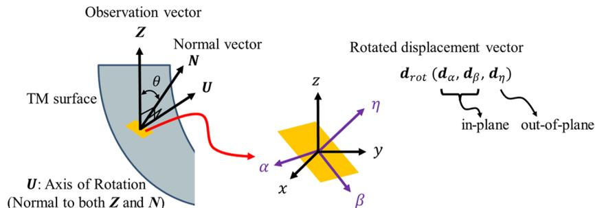
**Fig. 14** Transformation of the global measuring coordinate system  $x, y, z$  to the local coordinate system  $\alpha, \beta, \eta$ , of the TM. The observation vector  $\mathbf{Z}$  is rotated  $\theta$  degrees along the axis of rotation  $\mathbf{U}$ .
