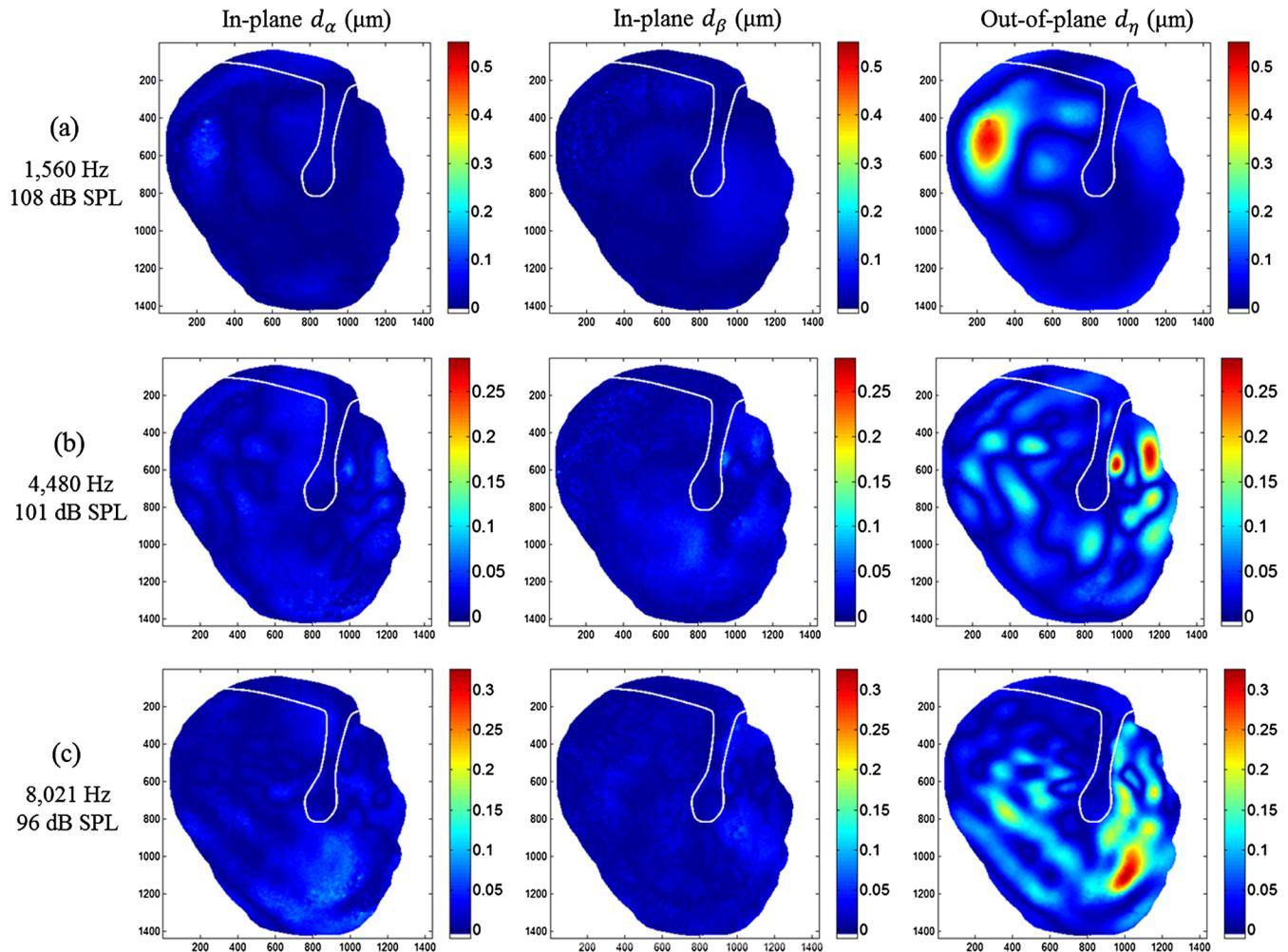
**Fig. 13** In-plane and out-of-plane sound-induced motions of a human TM excited with frequency of (a) 1560 Hz at 108 dB SPL, (b) 4480 Hz at 101 dB SPL, and (c) 8021 Hz at 96 dB SPL. It can be clearly seen that tangential (in-plane) components are negligible and the motions are mainly normal (out-of-plane) to the TM surface. Displacements are in the unit of micrometers.
