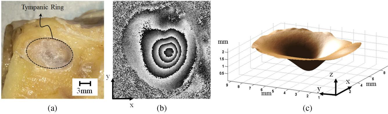
**Fig. 11** Measuring the shape of a human tympanic membrane (TM) using dual-wavelength holographic contouring: (a) human temporal bone highlighting the tympanic ring, (b) wrapped optical phase corresponding to the shape of the TM, and (c) 3-D shape of the TM. The shape is measured with wavelengths of 780.2 and 780.6 nm.
