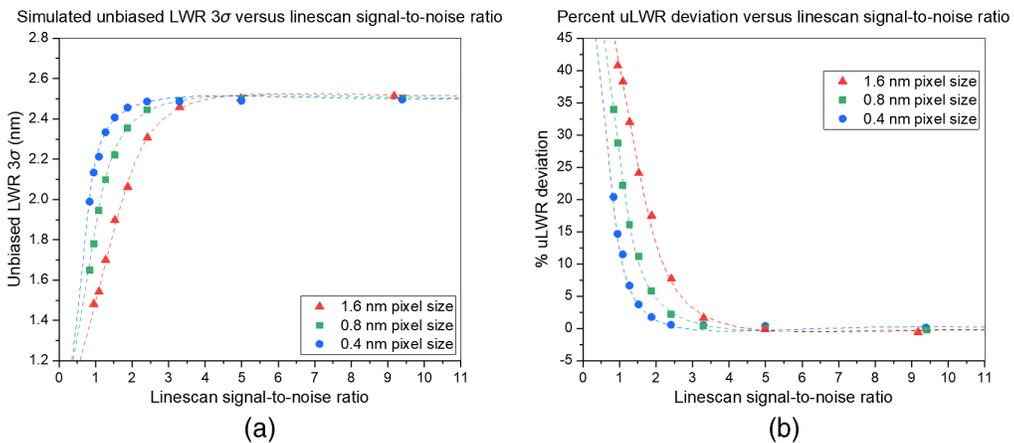
**Fig. 11** (a) Simulated unbiased LWR  $3\sigma$  for different pixel size with associated  $3\sigma$  standard deviation bars versus SNR and (b) uLWR percent deviation versus SNR of the synthetic SEM images.
