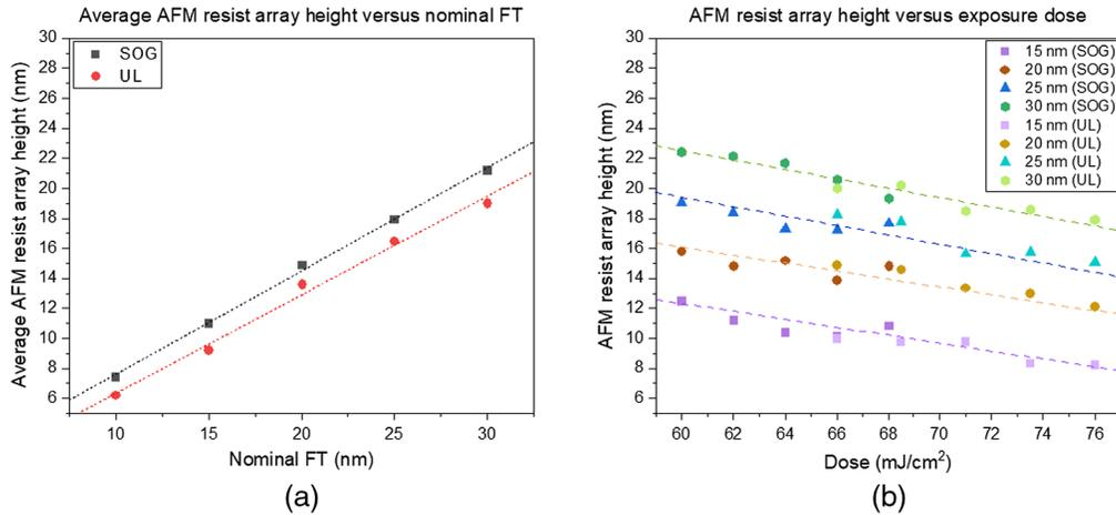
**Fig. 3** (a) Average AFM resist array height for five different dies through dose, and (b) the single AFM resist array height measurements for those dies plotted versus their respective exposure dose.
