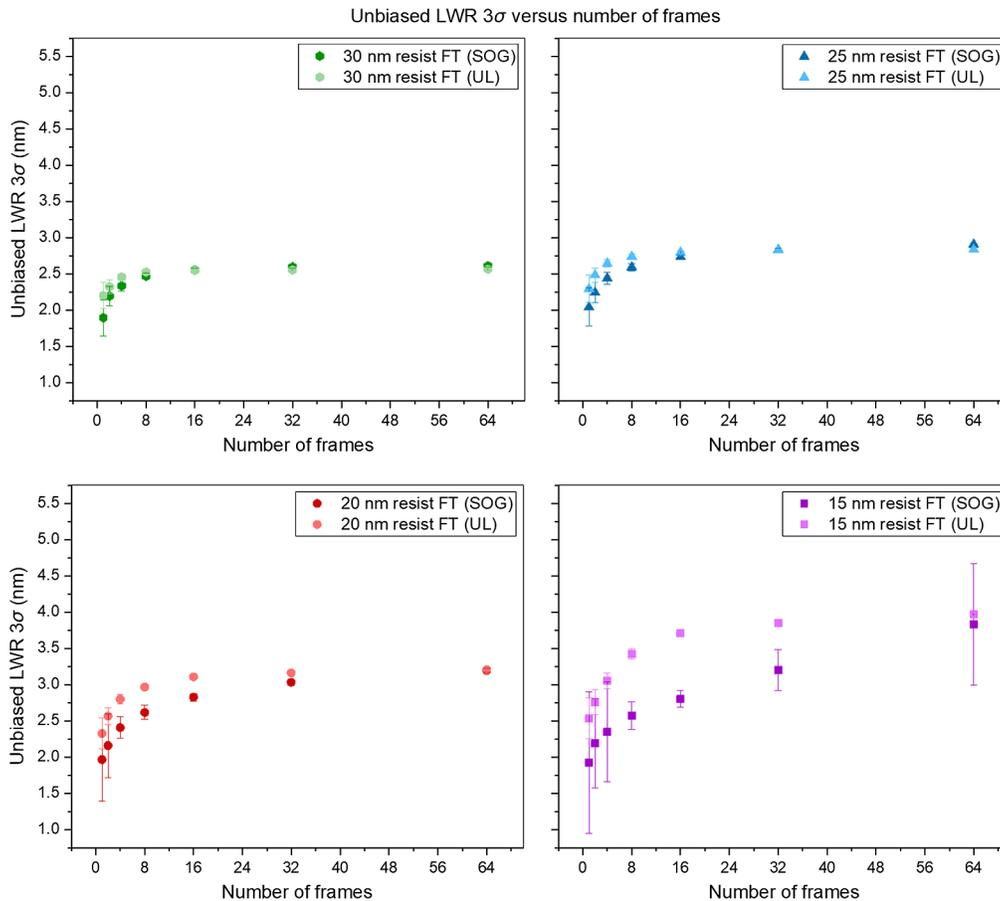
**Fig. 7** Unbiased LWR  $3\sigma$  versus a different number of frames (1, 2, 4, 8, 16, 32, and 64) for different resist FT variations with associated  $3\sigma$  standard deviation error bars determined from 50 images.
