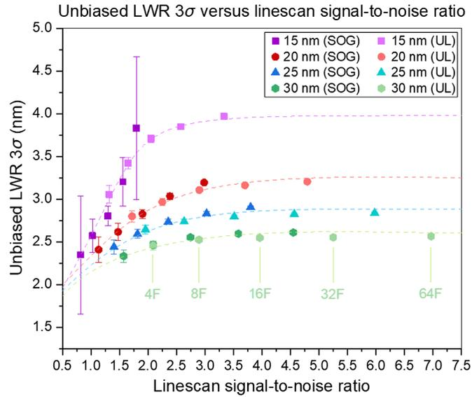
**Fig. 8** Unbiased LWR  $3\sigma$  versus SNR for different number of frames (4, 8, 16, 32, and 64) for different resist FT variations on SOG and UL with associated  $3\sigma$  standard deviation error bars determined from 50 images. An example for the different number of frames is given for 30 nm (UL).
