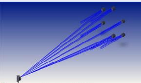
Ray tracing results when optical parameters are set in the FFSAT mechanical model. The rays are calculated results when observing a point light source on the optical axis and at infinite distance.
