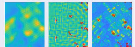
The left image shows a part of the synthetic aperture image. In the middle image is the reconstructed image after applying a high-pass filter. In this image, the region with a value larger than the reference value was extracted as the region with high spatial frequency. The position of the region is indicated by the red x symbol in the figure. In addition, the extracted positions are superimposed on the image of the large aperture single mirror to show the detection results.
