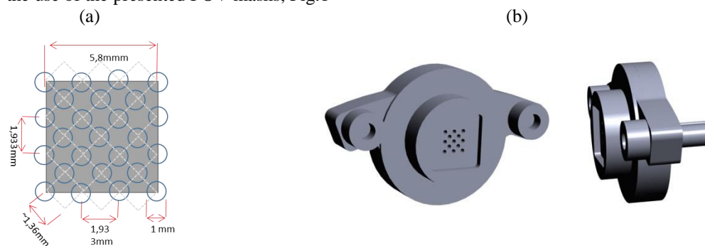
Fig.1: a)Distribution of drilled holes b) Optomechanical FOV masks employed for the RDS instruments.
