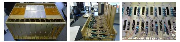
Fig. 11 : Interconnects of the optical plane to different slices of the breadboard
