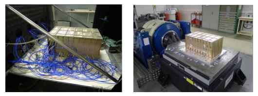
Fig. 12 : Optical interconnect breadboard under environmental test: thermal vacuum (left) and vibrations (right)
