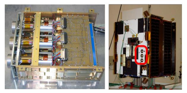
Fig. 1. LYRA instrument (left) and LYRA on the PROBA-2 spacecraft (right) Proc. of SPIE Vol. 10565 105650A-2
