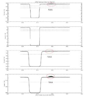
Fig. 2. First light sun pointing on head 2. The noisy data are observed on channel 2 and 4 of head 2. The small bumps are linked to spacecraft rotation. The spacecraft makes a  $90^{\circ}$  spin rotation 4 times per orbit
