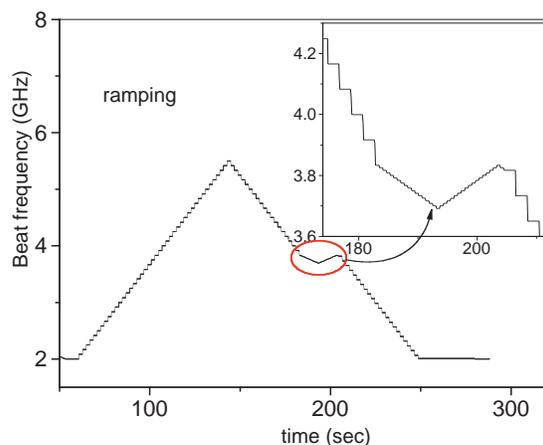
Fig. 5: Frequency tuning sequence, the insert shows the transition from coarse (83.33 MHz) to fine (8.333 MHz) frequency tuning steps (and reverse)
