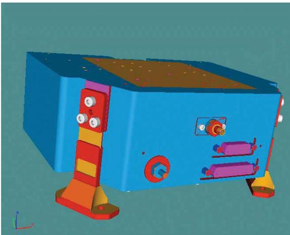
Fig. 6: RLH housing, showing isostatic mounts and connector interface.
