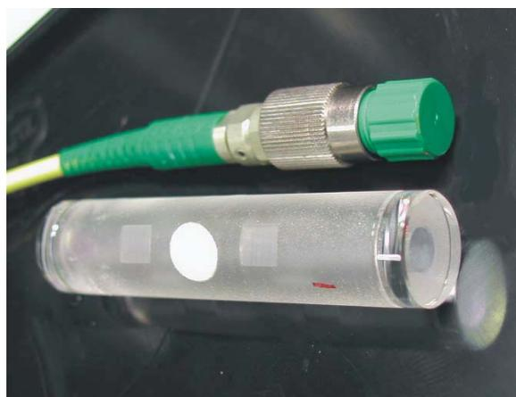
Fig. 3: ULE cavity in comparison with a FC/APC connector
