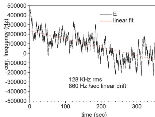
Fig. 4: First measurements of frequency stability of a RL locked to a cavity resonance.
