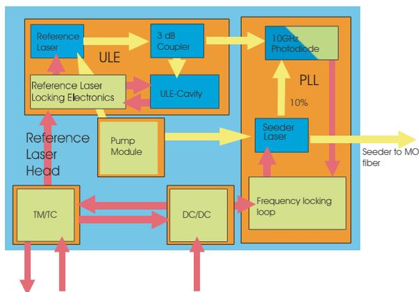
Fig. 2. Internal structure of RLH. Red arrows are electrical signals, yellow arrows are optical. Digital TM/TC is performed by a FPGA
