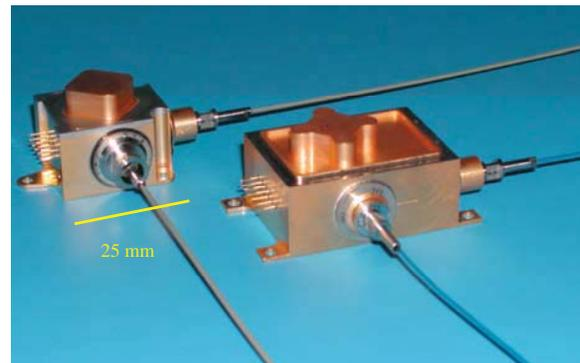
Fig. 1. TESAT single frequency Laser Heads
