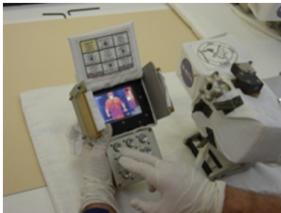
Figure 4. Infrared inspection system designed for on-orbit inspections.
