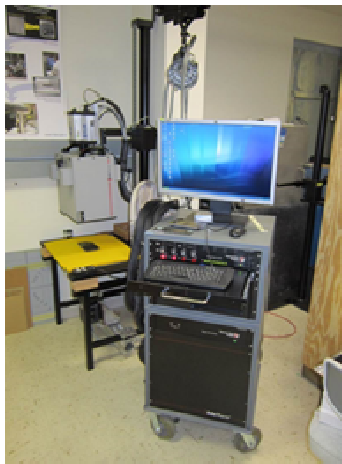
Figure 1. Photograph of the flash thermograph system.
