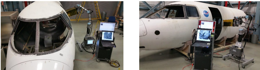
Figure 8. Two photographs of flash infrared thermography inspection performed on a composite aircraft fuselage by a cobot.
