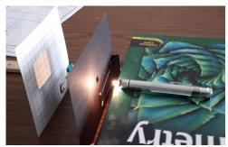
Figure 3 - Observing how light spreads from a "point" source. The light source was a MagLite<sup>®</sup> flashlight in candle mode. Binder clips were used to hold the mask and screen vertical.
