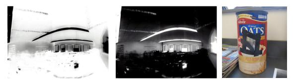
Figure 2 - Roughly 30 minute oatmeal box pinhole camera exposure of classroom (left), inverted version (center) and oatmeal box camera (right).
