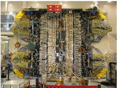
Figure 6 Typical Payload Panel Equipment Layout (Eurostar E3000 Platform) using conventional RF equipment. <sup>[19]</sup>. Imagine 1000 optical fiber and connectors binding modules on that scale.
