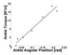
Fig. 2. Ankle torque versus position data for a normal subject walking on a horizontal surface. Only ankle data during the controlled plantarflexion phase of walking are shown. Although data for just one subject and one walking step are plotted, the human ankle behaves like a linear spring throughout early stance independent of walking speed, storing and releasing energy, and allowing for a smooth heel to forefoot strike sequence.<sup>26</sup>
