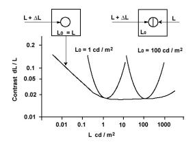
Fig. 4. The effect of luminance on contrast sensitivity The arrangement of the test field shown on the left is used to measure the absolute contrast sensitivity. The test field arrangement shown on the right is closer to a real image where the average luminance may vary widely from place to place.
