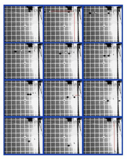
Figure 2 Elastic impact of two metal spheres.
