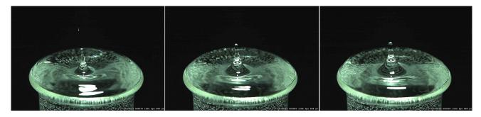
Figure 3 Surface tension behavior of water or simply falling water drops on water surface recorded by 1500 fps. Between the first (Frame 76) and the second picture (Frame 85) are 5976  $\mu$ s and between the second and the last picture (Frame 93) are 5312  $\mu$ s. (© D. Curticapean - Offenburg University)
