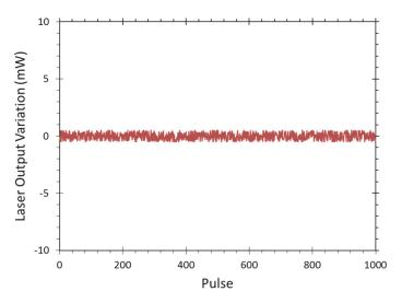
**Figure 4.3** A wasted graph. The *y* axis is chosen to give the impression that the there is little variation in the output, but if we cannot see any variation in the data, why show the graph?
