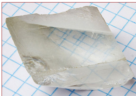
FIGURE 1.7.1 Ordinary and extraordinary component of light while passing through an anisotropic material. Dual image effect.
