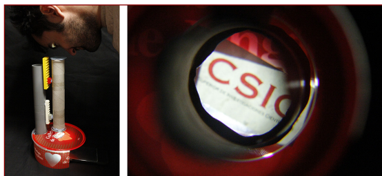
FIGURE 3.8.2 Final view of the built microscope, which shows how the object is illuminated with the flashlight of a mobile phone and imaged through the system.
