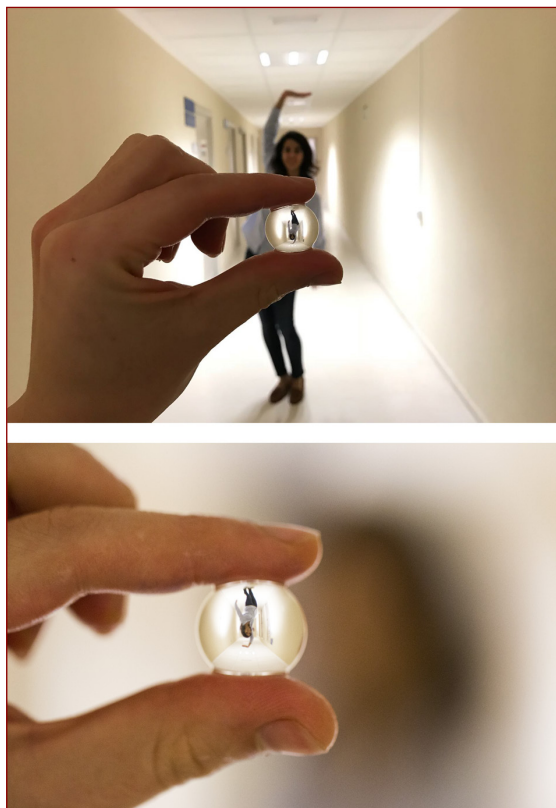
FIGURE 3.4.3 Formation of an inverted image of a distant object with a hydrated hydrogel pearl.
