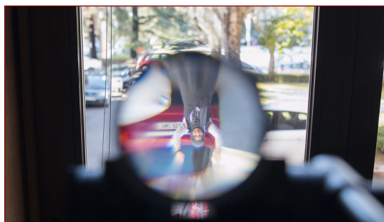
FIGURE 3.7.5 Inverted image produced by the Kepler telescope.
