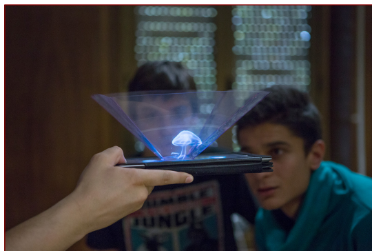
FIGURE 3.1.4 Photo of the pseudo-holographic pyramid. Photography: Juan Aballe / Scientific Culture (CSIC) / IOSA.
