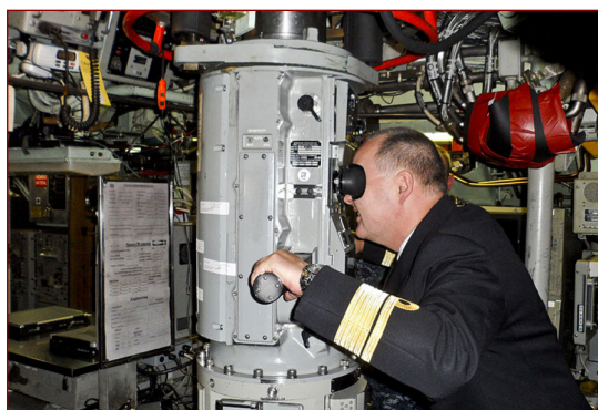
FIGURE 3.2.1 A periscope inside an American navy submarine.
