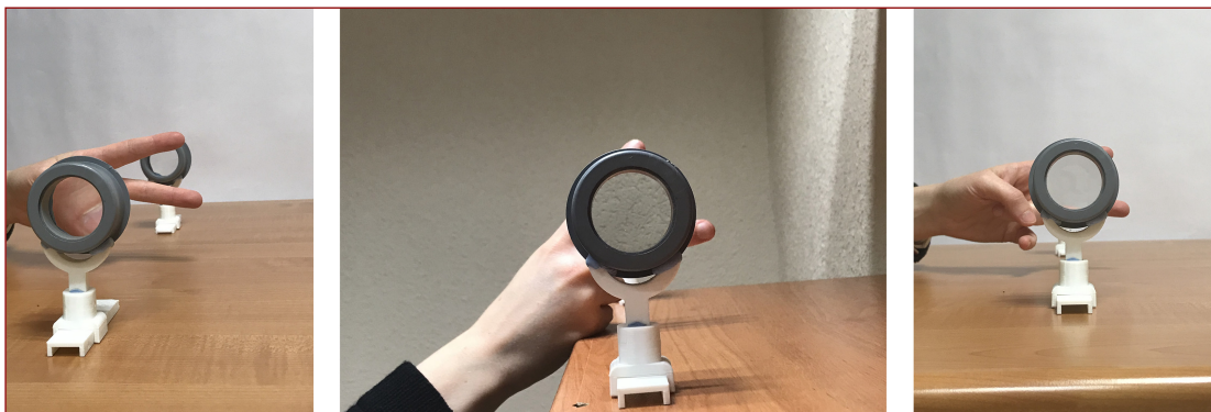
FIGURE 3.5.5 Assembly and proof of invisibility with lenses.
