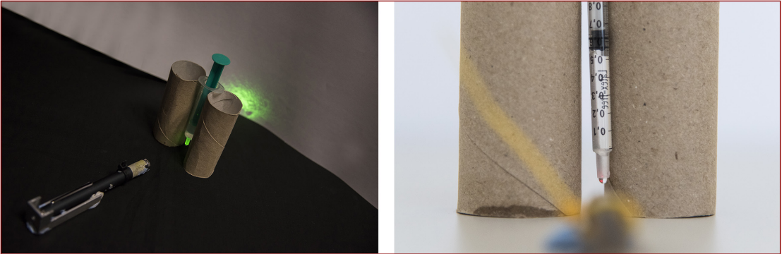
FIGURE 3.9.2 Assembly of the complete experiment (left) and detail of the assembly in which the suspended droplet (right) is observed.
