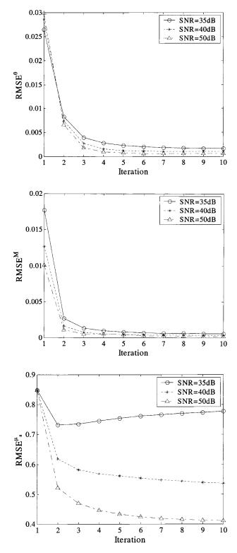
Fig. 5 Iteration vs three types of RMSE plots with differing SNR in the excitation wavelength.
