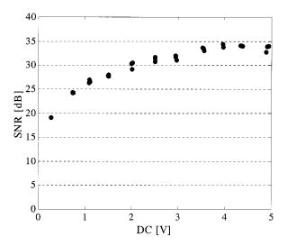
Fig. 3 SNR as a function of source dc power at the emission wavelength.
