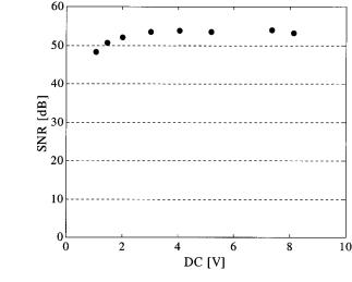
Fig. 2 SNR as a function of source dc power at the incident wavelength.
