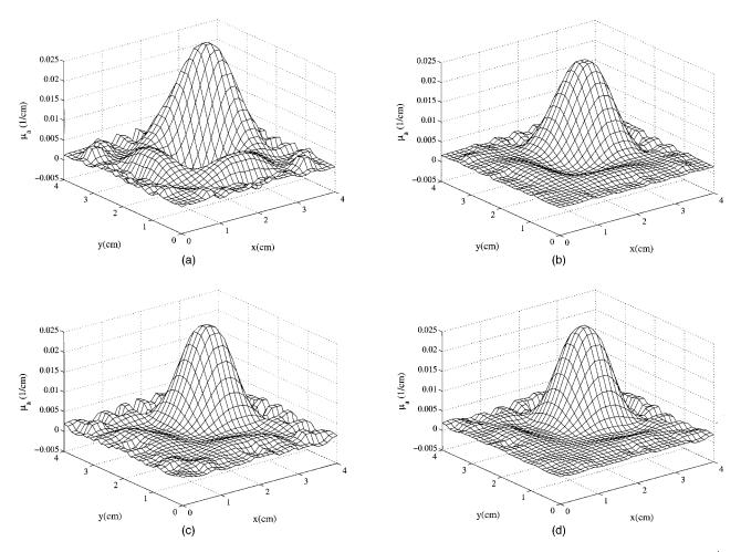
**Fig. 6** Reconstruction of  $\mu_{ax \to m}$  with the emission wave at various levels of SNR. The modulation frequency is set to 100 MHz, and  $\mu_{ax \to m}^b = 0.002 \text{ cm}^{-1}$ ,  $\mu_{ax \to m}^{\text{hetero}} = 0.02 \text{ cm}^{-1}$  (10:1 uptake ratio),  $\mu_s^x = \mu_x^m = 10 \text{ cm}^{-1}$ , lifetime of both heterogeneity and background are set to 0.58 ns. The regularization parameter  $\lambda$  is set to  $10^{-7}$  for (a) and (b), and  $10^{-8}$  for (c) and (d).
