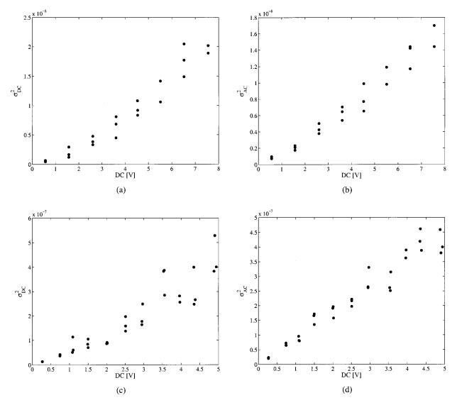
**Fig. 8** (a) Standard deviation of detected dc vs dc power of source, (b) standard deviation of ac amplitude vs dc power of source at incident wavelength, (c) standard deviation of detected dc vs dc power of source, (d) standard deviation of ac amplitude vs dc power of source at the emission wavelength.
