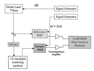
Fig. 1 Schematic diagram of the experimental setup for frequency domain photon migration measurements.
