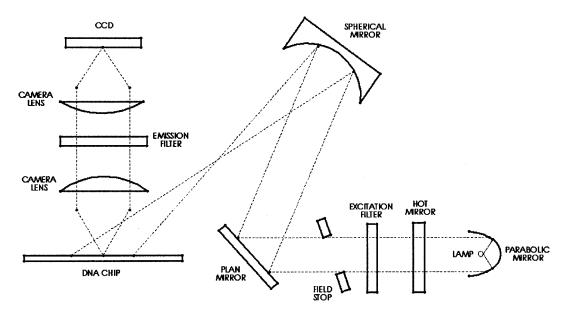
Fig. 1 Optical layout of the imaging system.
