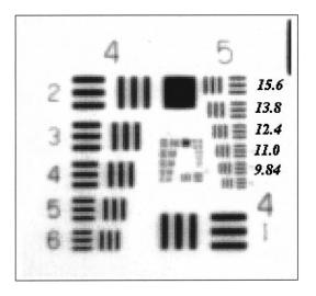
**Fig. 2** Image of positive standard USAF 1951 resolution test pattern. Italic numerical values indicate the linewidth for the adjacent elements in group 5.
