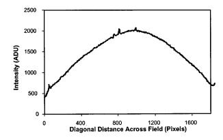
**Fig. 3** Overall shading effect due to illumination inhomogeneity and imaging aberrations, showing the pixel intensity along the diagonal line of the image of a plastic filter. The image was acquired with excitation centered at 570 nm.
