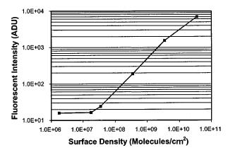
Fig. 5 Plot of measured fluorescence intensity vs surface density of SpectrumRed molecules.
