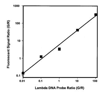
**Fig. 6** Dynamic range of the assay system. Denatured doublestranded lambda target DNA was deposited on chromium chips (80 spots per array). Lambda probe DNA was labeled by nick translation. Each hybridization reaction contained a mixture of 250 pg of SpectrumRed lambda DNA and either 2.5 pg, 25 pg, 250 pg, 2.5 ng, or 25 ng of SpectrumGreen lambda DNA. The average green/red intensity ratios are plotted vs the concentration ratio of green/red probe DNA.
