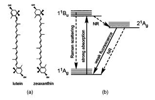
**Fig. 1** (a) Chemical structure of lutein and zeaxanthin molecules. They differ in the location of the additional C=C bond in one ionone ring. (b) Energy-level diagram of long-chain carotenoid molecules with optical and nonradiative transitions.
