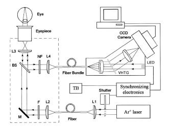
**Fig. 4** The setup of the fiber-based MP Raman detector, an instrument for quantitative measurements of macular carotenoid pigment content in clinical settings.
