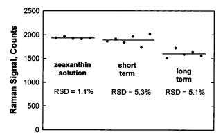
Fig. 11 Repeatability of Raman measurements. The left part represents data for zeaxanthin solution in a model eye. The central and right data represent the short-term and long-term repeatability of macular pigment measurements for two different subjects. The Raman intensities for the long-term dataset were measured over a 2-week period in five sessions.
