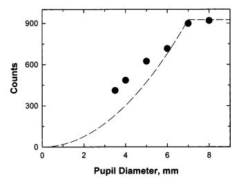
**Fig. 9** Measured variation in the Raman signal with pupil diameter for a human subject (circles). The dashed curve is the theoretically expected change in the signal with pupil diameter. Above a 7-mm pupil diameter, the signal stays constant (see text).
