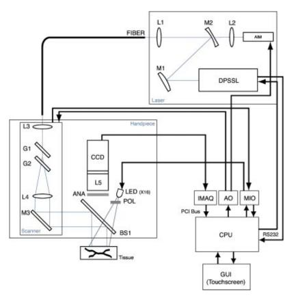
Fig. 2 System schematic.
