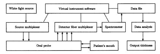
Fig. 12 Block diagram of oral DRS device showing how white light is transmitted to the patient and the reflected light is processed into a measure of epithelial thickness.
