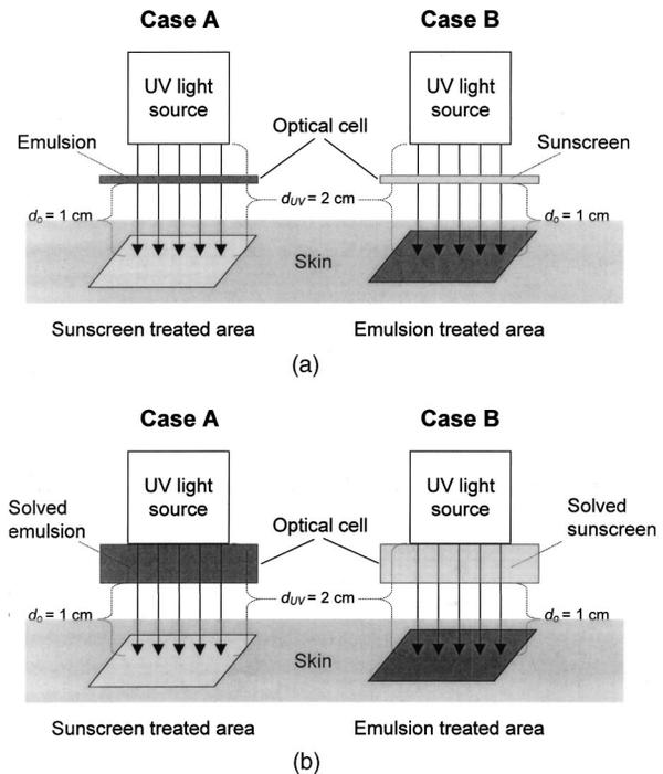
**Fig. 1** Arrangement for the determination of the SPF. (a) Protocol 1: direct application, cell length  $d=1$  mm. (b) Protocol 2: dissolved form, cell length  $d=1$  cm.
