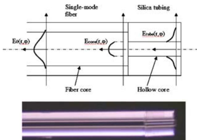
Fig. 1 Split wavefront IFPI sensor head structure.
