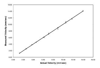
Fig. 2 Actual versus measured velocities of *in vitro* calibration wheel with error bars.
