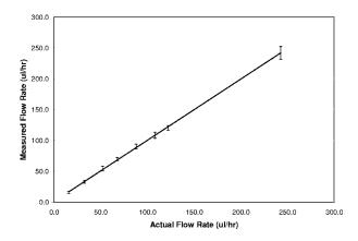
Fig. 3 Actual versus measured volume flow rates of microspheres flowing through  $140-\mu m$  glass tube.
