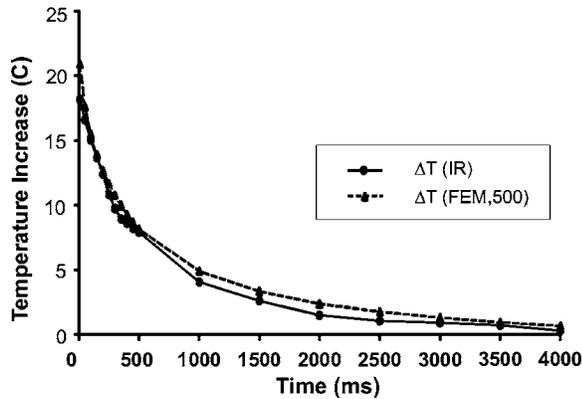
**Fig. 6** Comparison between computed (upper-faced solid triangle) and measured (circle) time-dependent temperature relaxations (wavelength of 1314 nm, at the center of the beam,  $h=500\text{ W/m}^2\text{K}$ ,  $D=1.3\text{ mm}$ ).
