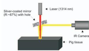
Fig. 2 Experimental setup for thermal dynamics imaging experiment.
