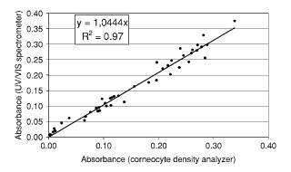
Fig. 4 Correlation between the pseudoabsorption determined by the modified UV/VIS spectrometer Lambda 20 and the corneocyte density analyzer.
