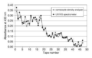
**Fig. 3** Pseudoabsorption of the tape strips determined by the modified UV/VIS spectrometer Lambda 20 and the corneocyte density analyzer.
