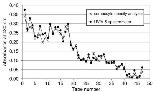
Fig. 3 Pseudoabsorption of the tape strips determined by the modified UV/VIS spectrometer Lambda 20 and the corneocyte density analyzer.
