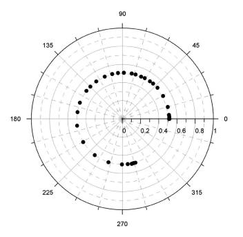
**Fig. 2** Operation curve provided by the TNLCD in the phase-only configuration. The points correspond to different gray levels sent to the device. The radial coordinate is the fraction of transmitted irradiance, and the polar angle is the phase retardation.
