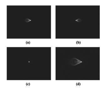
**Fig. 4** Compensation of the aberration  $Z_3^1$ : (a) aberrated PSF produced by the plate, (b) PSF produced by the SLM alone when encoding the four-level compensating phase, (c) PSF of the aberrated eye after compensation using the SLM, and (d) PSF of the aberrated eye when the SLM encodes an aberration of the same magnitude and sign as that of the plate, doubling in this way the original aberration.
