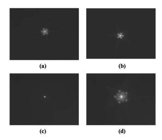
**Fig. 5** Compensation of the aberration  $Z_{5}^{5}$ : (a) aberrated PSF produced by the plate, (b) PSF produced by the SLM alone when encoding the four-level compensating phase, (c) PSF of the aberrated eye after compensation using the SLM, and (d) PSF of the aberrated eye when the SLM encodes an aberration of the same magnitude and sign as that of the plate, doubling in this way the original aberration.
