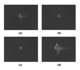
**Fig. 6** Compensation of a complex aberration pattern typical of a human eye: (a) aberrated PSF produced by the plate, (b) PSF produced by the SLM alone when encoding the four-level compensating phase, (c) PSF of the aberrated eye after compensation using the SLM, and (d) PSF of the aberrated eye when the SLM encodes an aberration of the same magnitude and sign as that of the plate, doubling in this way the original aberration.
