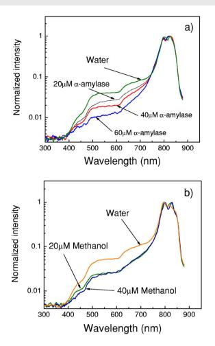
**Fig. 1** (a) White light spectrum of pure  $H_2O$  and  $H_2O + \alpha$ -amylase. Note the suppression of white light as the protein concentration is increased. For  $60-\mu M$  concentration, the suppression factors at 500 and 600 nm were 3.4 and 3.2, respectively. The incident 820-nm light had a spectral bandwidth of 30 nm. (b) White light spectrum obtained when methanol, an electron scavenger, is added to water.
