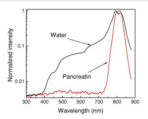
**Fig. 3** White light spectrum obtained with pure  $H_2O$  and  $H_2O$  + pancreatin. The white light suppression factors at 500 and 600 nm were 8.3 and 13.3, respectively.
