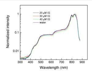
**Fig. 2** White light spectrum obtained with pure  $H_2O$  and  $H_2O$  + immunoglobulin (IG) at an incident laser intensity of ~1 TW cm<sup>-2</sup>. For 40- $\mu$ M concentration, the suppression factor was 2.1 at 500 and 600 nm. Similar results were obtained with lysine and arginine.
