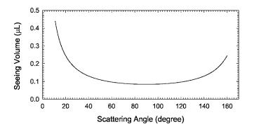
**Fig. 2** Calculated sample volume "seen" by the detector versus the scattering angle  $\theta_s$ .
