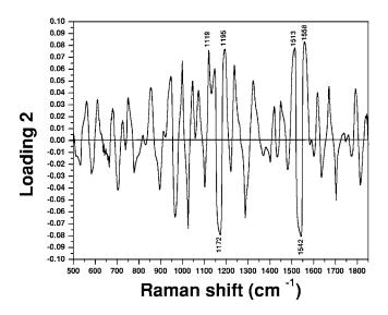
**Fig. 5** One-dimensional loading plot of PC2; the peaks with highest amplitude show the positions of the principal differences between positive and negative samples.
