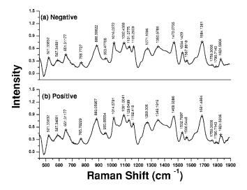
Fig. 2 Mean RS of (a) negative and (b) positive samples of human colostrum in the range from 450 to 1900 cm<sup>-1</sup>.
