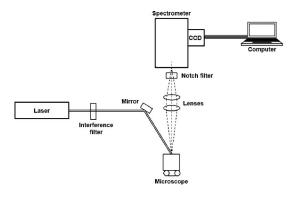
Fig. 1 Schematic diagram of the experimental setup of Raman spectroscopy.
