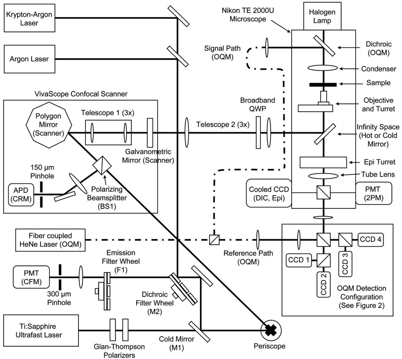
Fig. 1 Design of the multimodal optical microscope. Details are given in the text.
