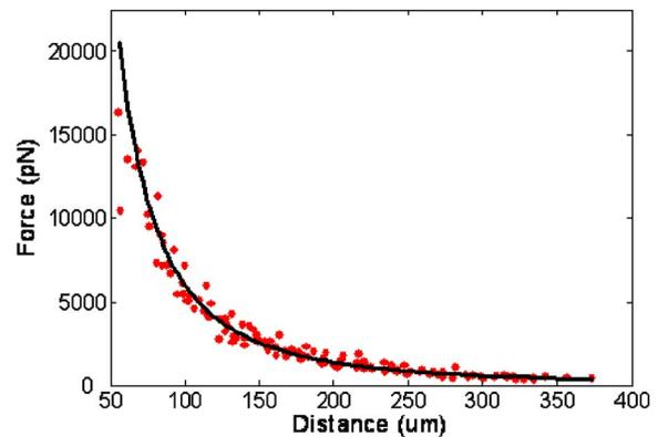
**Fig. 4** Force calibration results for a coil current of 0.05 A. This analysis allows for the electromagnet to be appropriately positioned to deliver the desired force to the cell. We specifically chose this current to place our desired force, 500 pN, on the flat portion of the curve to prevent slight variations in magnet position from introducing a significant amount of error in the applied force. This force was not achievable in previous studies using laser tweezers.<sup>15-17</sup>
