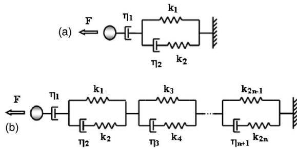
**Fig. 1** (a) A commonly used mechanical model for the cytoskeleton consists of a standard linear solid (SLS) body in series with a dashpot. This model represents changes within the cell as a force,  $F$ , is applied to an attached magnetic bead. It produces a fast elastic and slower viscous behavior, as seen in Eq. (1). (b) These types of models can be extended to include multiple time constants by adding additional SLS bodies [Eq. (2)].
