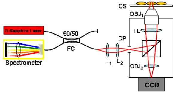
**Fig. 5** SDPM common-path implementation adapted to an inverted microscope. Source light from a Ti:Sapphire laser passes through a 50/50 fiber coupler (FC). The beam is relayed into the microscope via a documentation port (DP). System components include the spectrometer (Spect.), collimating lens ( $L_1$ ), SDPM objective lens ( $L_2$ ), tube lens (TL), microscope objective ( $OBJ_1$ ), coverslip (CS), camera objective ( $OBJ_2$ ), and camera (CCD).
