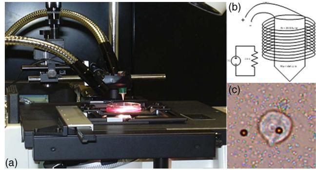
**Fig. 3** (a) Experimental setup showing the electromagnet mounted above the cell sample. The tip of the magnet was within the media during actual experiments. (b) Electromagnet schematic. (c) Photomicrograph of an MCF-7 cell with fibronectin-coated magnetic bead attached.
