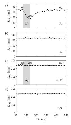
**Fig. 5** Gas exchange study for the right maxillary sinuses using detection geometry *PC* on volunteer 1 (see text). (a)  $L_{eq}$  for oxygen (solid dots) measured as a function of time with N<sub>2</sub> flushing, together with a line drawn for guidance of the eye (dashed line). (b) Same as (a) without N<sub>2</sub> flushing. (c)  $L_{eq}$  for water vapor (solid dots) measured as a function of time with N<sub>2</sub> flushing. (d) same as (c) without N<sub>2</sub> flushing.
