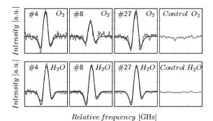
**Fig. 6** Balanced detection signals measured for oxygen and water vapor during the gas exchange study using detection geometry *PC*. The numbers correspond to the ones indicated in Fig. 5. The relative frequency range is about 30 GHz. The control signals are also shown for both gases when measuring through the cheek.
