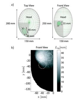
**Fig. 3** (a) A model used for Monte Carlo simulations created in ASAP<sup>TM</sup> representing measurements on the human maxillary sinus according to detector geometry *PC*. The region where the rays were collected is indicated by the gray shaded area. The cross represents the location of the light source. (b) The simulated  $L_{eq}$  for the model shown in (a). The different positions of the detector in the case of real measurements are also indicated.
