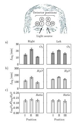
**Fig. 9**  $L_{eq}$  for (a) molecular oxygen and (b) water vapor measured in left and right frontal sinuses for volunteer 1 using detection geometry *OF* and detection positions according to the top figure. The data shown correspond to the average of ten recordings together with two standard deviations. (c) The ratios of the  $L_{eq}$  for oxygen and water vapor are shown.
