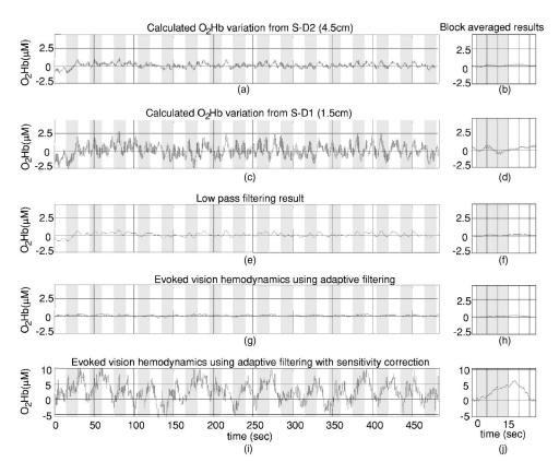
**Fig. 3** Adaptive filtering to remove global interference and recover evoked brain activity. (a) Target  $O_2Hb$  measurements from S-D2 with 4.5-cm source-detector separation, and (b) its block averaged result. (c) and (d) Reference measurements from S-D1 with 1.5-cm source-detector separation. (e) and (f) Low-pass filtering result for the target measurements. (g) and (h) Adaptive filtering result for the target measurement. (i) and (j) Adaptive filtering result with sensitivity correction.
