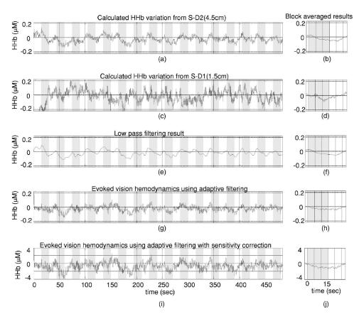
**Fig. 5** Adaptive filtering to remove global interference and recover evoked brain activity. (a) Target HHb measurements from S-D2 with 4.5-cm source-detector separation, and (b) its block averaged result. (c) and (d) Reference HHb measurements from S-D1 with 1.5-cm source-detector separation. (e) and (f) Low-pass filtering result for the target measurements. (g) and (h) Adaptive filtering result for the target measurement. (i) and (j) Adaptive filtering result with sensitivity correction.
