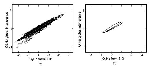
Fig. 8 (a) Linear regression between the global interference in  $O_2Hb$  from S-D2 (vision response subtracted) and  $O_2Hb$  from S-D1. (b) A continuous plot of one 20-s segment. The arrow indicates the direction of change as a function of time.
