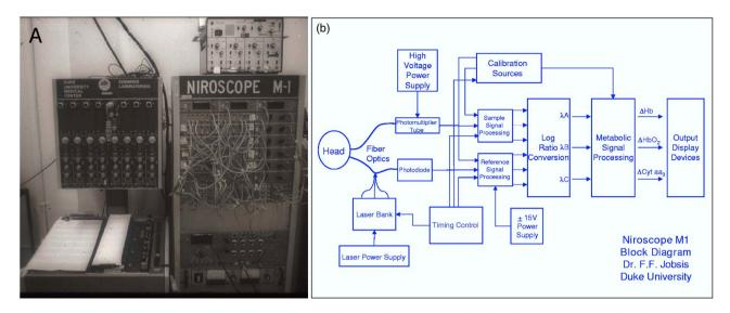
**Fig. 1** (a) Photograph of the first working prototype of the Jöbsis Niroscope circa 1982. (b) Early block diagram of a three wavelength instrument for monitoring a single tissue. The actual Niroscope prototype was a four wavelength instrument capable of monitoring two separate tissues simultaneously.
