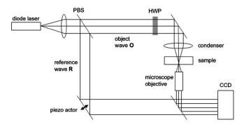
Fig. 1 Experimental setup for phase-shifting digital holography. PBS: polarizing beamsplitter; HWP: half wave plate.
