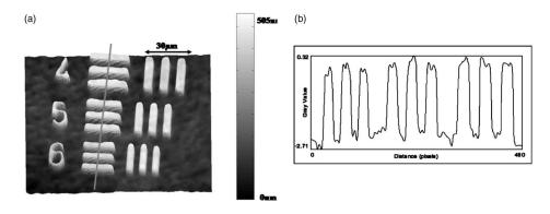
**Fig. 5** (a) Surface topology of the etched transparent reference chart (elements 4 to 6 of group 6) recorded by the digital holographic microscope, magnification  $20 \times$ ; (b) line scan of gray values as marked in the pseudo 3-D image.
