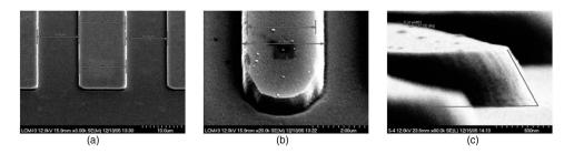
**Fig. 4** Scanning electron microscopy images of the etched reference chart: (a) Top view, element 4 of group 5, scale bar 10  $\mu$ m, top width 10.8  $\mu$ m, bottom width 11.9  $\mu$ m. (b) Top view, element 6 of group 7, scale bar 2  $\mu$ m, top width 2.54  $\mu$ m, bottom width 3.19  $\mu$ m. (c) Tilted view, scale bar 500 nm, angle between step and bottom 62 deg.
