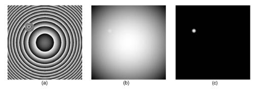
**Fig. 2** Unwrapping and fitting of a quadratic function illustrated on a simulated example. Image (a) represents a wrapped phase distribution, images (b) and (c) show the same image after unwrapping and subtracting a fitting quadratic function, respectively.
