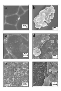
**Fig. 4** SEM images of PDLLA deposits at different magnifications: (a) and (b) PDLLA1, (c) and (d) PDLLA4, (e) and (f) PDLLA5.
