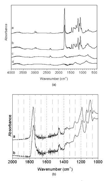
**Fig. 3** (a) FTIR spectra between 4000 and 400 cm<sup>-1</sup> of drop cast PDLLA (trace a), PDLLA5 (trace b), PDLLA4 (trace c), and PDLLA1 (trace d). (b) FTIR spectra of drop cast PDLLA (trace a) and PDLLA5 (trace b) between 2000 and 1000 cm<sup>-1</sup>.
