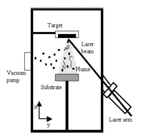
**Fig. 2** MAPLE setup, top view. The target movement is in the *yz* plane, where the *z*-axis is normal to the *xy* plane.
