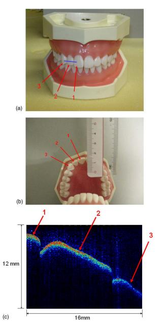
**Fig. 8** (a) Phantom seen from front. (b) Phantom seen from bottom. (c) OCT image of three phantom teeth.
