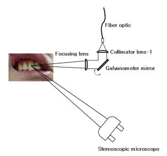
Fig. 3 Setup for *in vivo* imaging.
