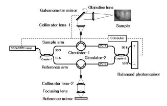
Fig. 1 Experimental setup of the OFDR-OCT system.
