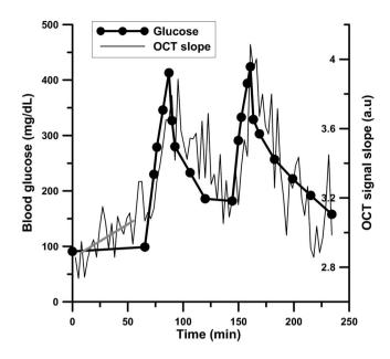
**Fig. 2** OCT signal slope and blood glucose concentration versus time when low pressure (<1 kPa) was applied on the skin by the OCT probe with the 50-mm adaptor.
