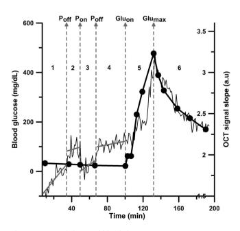
**Fig. 3** OCT signal slope and blood glucose concentration versus time when high pressure (intervals 1 and 3) and low pressure (intervals 2 and 4) were interchangeably applied on the skin by the OCT probe with the 50-mm adaptor. The measurements in intervals 5 and 6 were performed at low pressure. Glucose was injected during interval 5.
