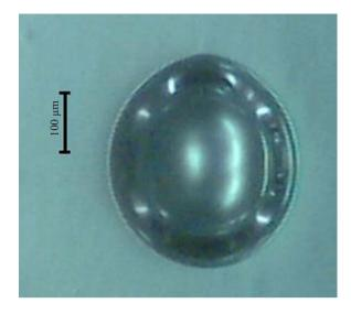
**Fig. 4** Optical image of a laser-induced cavitation bubble. The laser beam was delivered from the bottom and the ultrasound transducer was positioned at the top, as indicated in Fig. 1.
