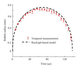
**Fig. 6** Measured (time-of-flight method) and modeled (cavity lifespan or collapse time and Rayleigh equation) dynamic behavior of cavities produced by the pulsed nanosecond laser. Only a subset of data corresponding to cavitation bubbles with a lifespan between 135 to 140  $\mu$ s was used. The error bars represent plus/minus one standard deviation of the estimates.
