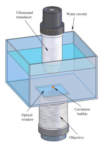
**Fig. 1** Schematic view of the experimental setup. The microbubbles were produced in a water cuvette using a 5-ns laser beam focused by an objective lens through the optical window at the bottom. The ultrasound transducer, positioned at the top, was aligned with the laser beam such that the cavity was located approximately at the focus of the transducer.
