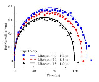
**Fig. 7** Comparison of measured (time-of-flight) and modeled (Rayleigh equation) temporal behavior of cavitation bubbles characterized by different lifespans.
