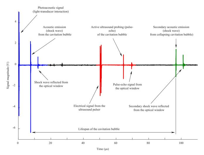
Fig. 2 Typical ultrasound RF data record containing both passive and active acoustic signals that correspond to initial cavity formation, ultrasound pulse-echo probing of the bubble, and bubble collapse.
