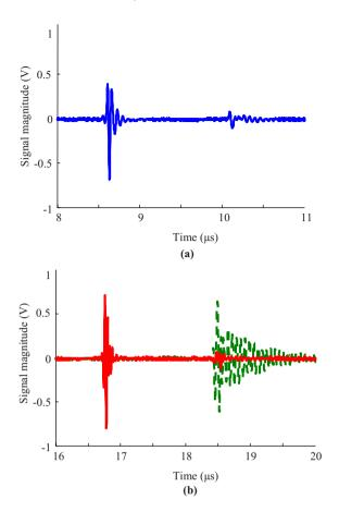
**Fig. 5** Temporal characteristics of (a) passive acoustic emission from the cavity, and (b) pulse-echo ultrasound probing of the cavitation microbubble (solid line). Prior to the experiment, the echo signal from the optical window at the bottom of the cuvette was captured [dashed line in Fig. 5(b)]. These acoustic signals were used to determine the radius of the microbubble at equilibrium.
